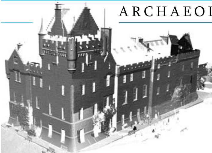
A three-dimensional model of Brodick Castle based on laser survey imagery
